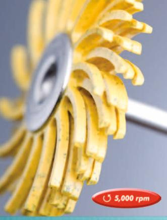
**HABRAS Disc Pro** are brush shaped mounted polishing discs. They consist of soft polyamide in which abrasives are embedded. The unique brush design of these discs and their colour indicated abrasiveness enhance their effectiveness. From fine grinding, through pre-polishing up to fine polishing, these **HABRAS Disc Pro** have many applications. **HABRAS Disc Pro** are used at 5,000 rpm without any additional polishing compound.
