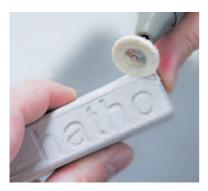
Ideal results are gained using 10.000 rpm's and using our novel polishing compound (Polistar lintygrey).
