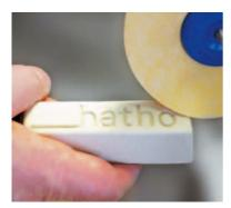
The prosthesis now has an even surface and is ready for first stage polishing.
