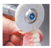
The narrow goat hair brush (*ArtNo. 100 48*) gets into hard to reach areas such as interproximal areas, gingival margins, palate wrinkles and the finishing line between metal and acrylic in combined cases with partial frameworks. To reduce heat development, 1400 rpm's have proven to give the best results. The acrylic surface is now ready for the final stage, polishing to a high shine.
